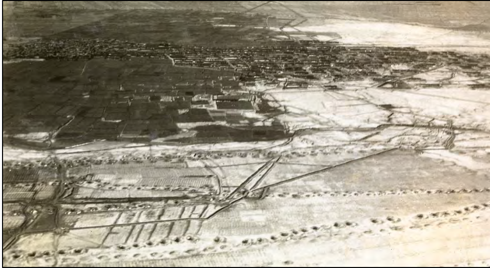
Esfahan, qanat access shaft mouths at Kashan, February 1925 (CC0, cropped and sharpened, ETH-Bibliothek, Walter Mittelholzer).
